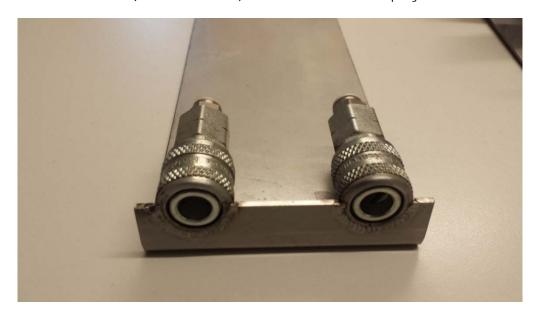
Attachment to Aircraft – In simple, the Pilot/Flight Crew or Fire Fighters simply attach the HELiFIRE Monsoon Bucket to the Helicopter hook, then they plug in the ARO quick release bayonet connectors to the source of air. They then connect the HELiFIRE Dump System Controller to an existing 24-volt dc power source on board the Helicopter...and you are ready for operation.
